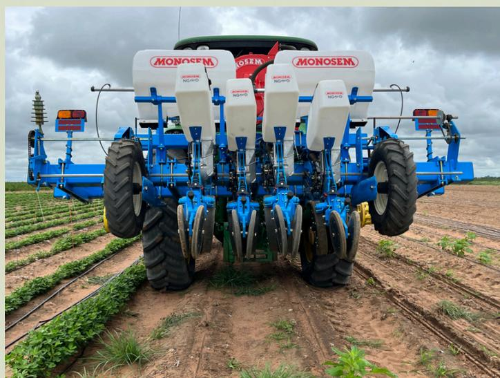
**Figure 1:** Monosem precision planter used for sowing Kalonji on 30 cm row spacing in Emerald, QLD.
