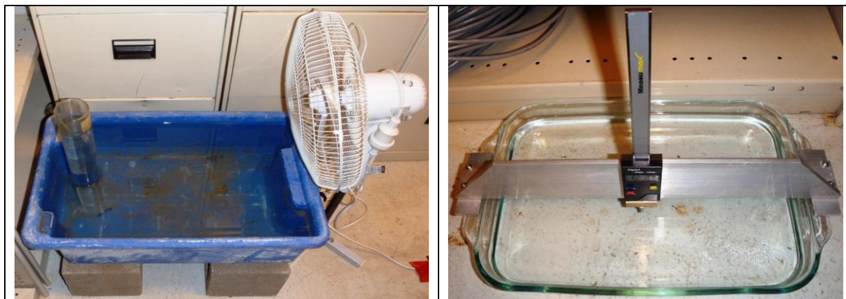
Figure 2 – (A) Example fan and tank configuration. The large graduated tube placed in the left hand side of the tank was used to make a simple estimate of the water level before and after each experiment. (B) Standard/control evaporation measurement container (clear glass) on top of which sits a fixed digital distance gauge.
