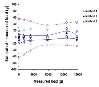
**Figure 1.** Variation in deviation of estimated load from measured load for selected load cells as a function of measured load with three methods of estimation. Dashed line indicates the upper and lower boundaries of the deviation of load as a function of measured load for method 1 and the solid line shows the boundaries of combined deviation for methods 2 and 3.
