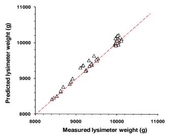
**Figure 3.** Variation in predicted lysimeter weight (with the 6-point calibration method) over the range of measured lysimeter weights. The dashed line represents the 1:1 line.
