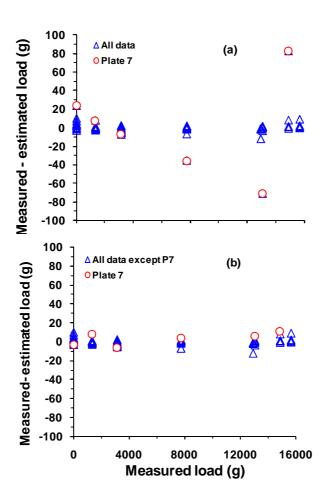
**Figure 2.** Variation in deviation of estimated load from measured load over the range of measured loads for all load cells using a 6-point calibration equation (a) without minimisation of deviation for Plate 7 (load cell 7) and (b) after minimisation of deviation for Plate 7. Dashed line indicates the line of zero deviation.
