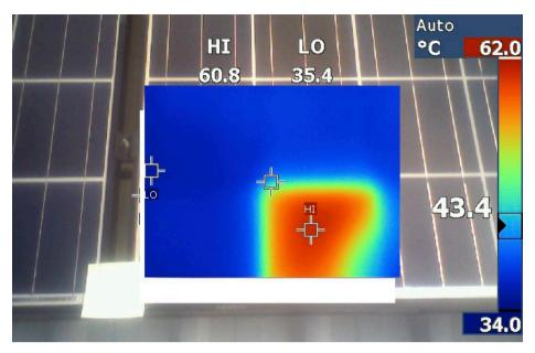
Figure 1: USQ is experimenting with using infrared thermal images to detect PV faults. This image from a USQ student's research shows how hot spots can be detected; this is made simpler in the USQ solar car park as they can be detected from underneath the structure.
