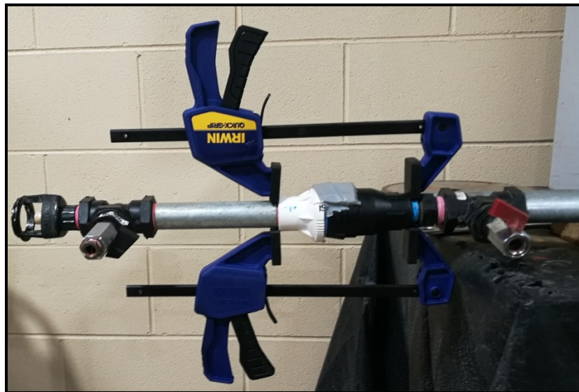
Figure 4-13: Set-up of manufacturer Y pressure regulator during low head testing
