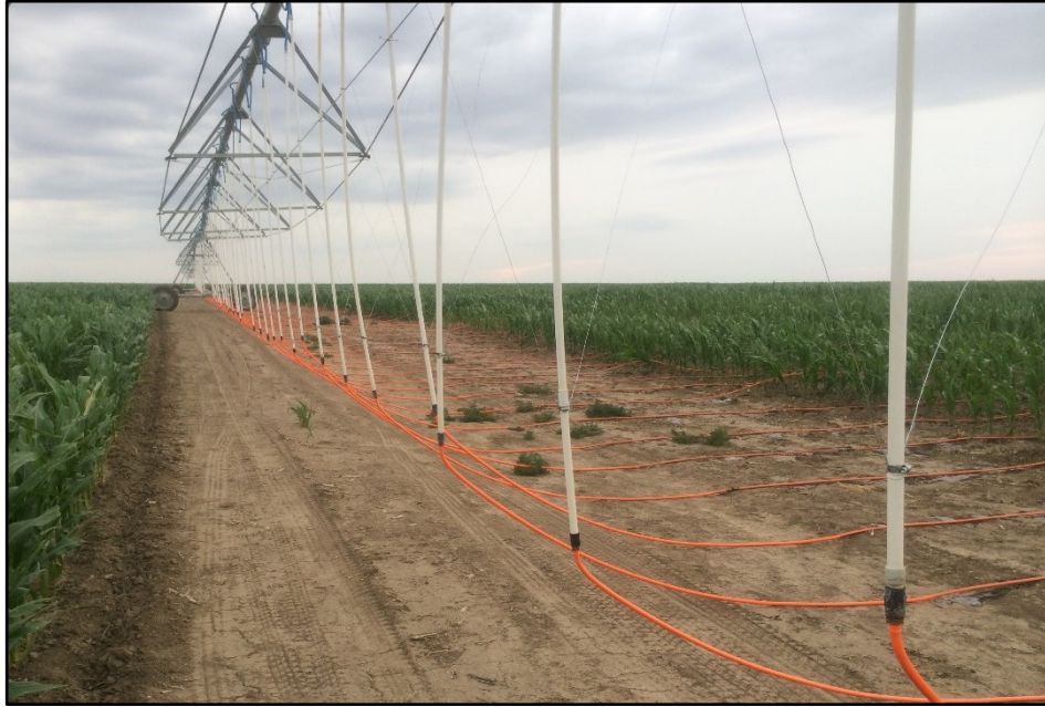
Figure 1-4: Precision Mobile Drip Irrigation (PMDI) technology with CP&LMs
