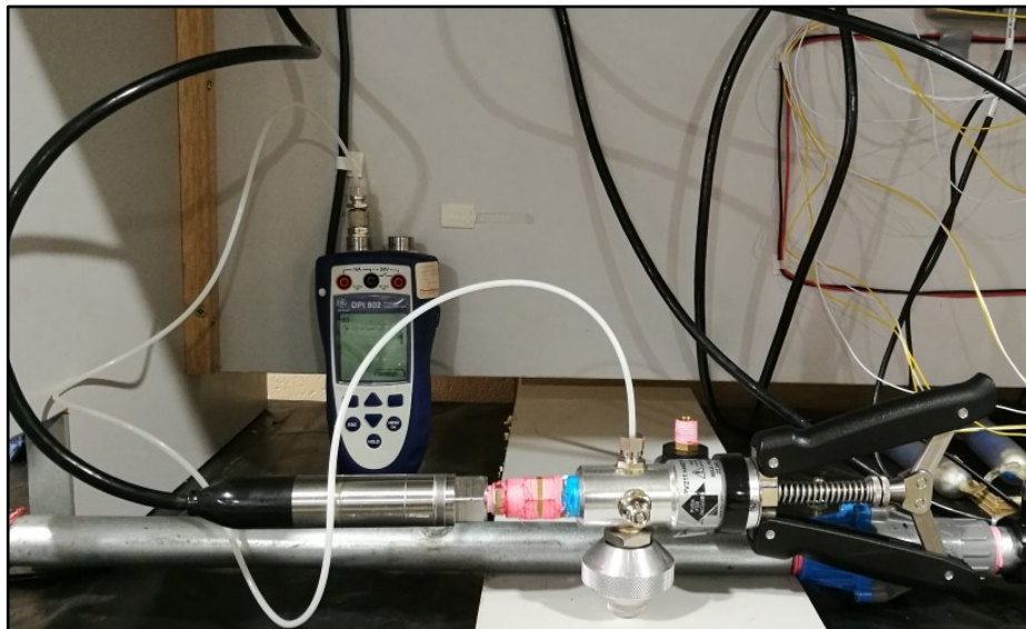
Figure 4-1: Calibration of pressure transducers using a Druck PV211 pneumatic pressure hand pump with a Druck DPI 802
