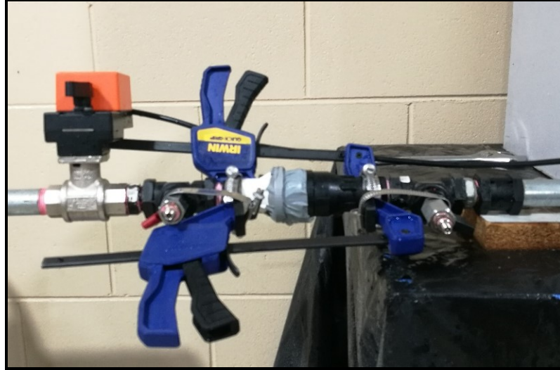
Figure 4-12: Set-up of manufacturer Y pressure regulator during minor head loss testing at Z113 Hydraulics Laboratory
