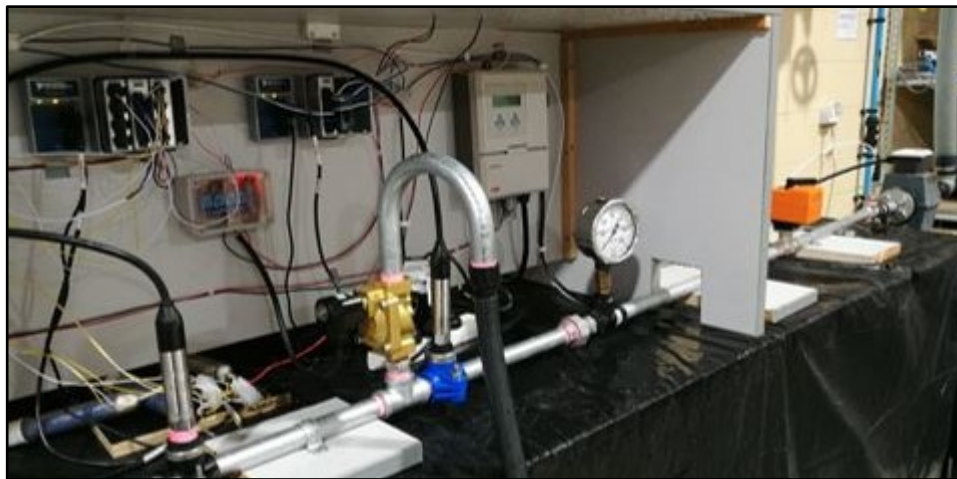
Figure 4-4: “Configuration B” of the VRI valve installation in the test apparatus connected to a 10 psi regulator via a gooseneck and fibre reinforced drop hose
