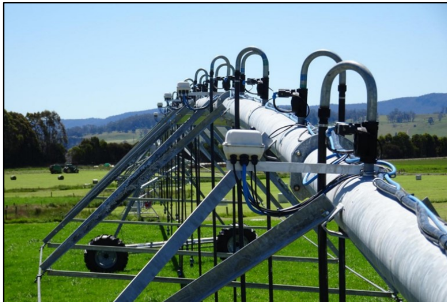
Figure 1-3: Configuration of VRI sprinkler solenoid valves in the lateral of CP&LMs (Foley, 2015)
