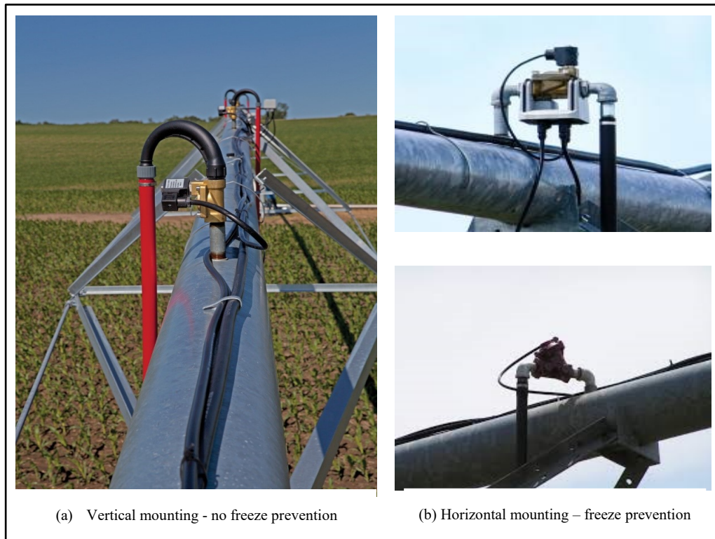
Figure 1-6: VRI valve configurations for CP&LMs in cold and warm temperatures
