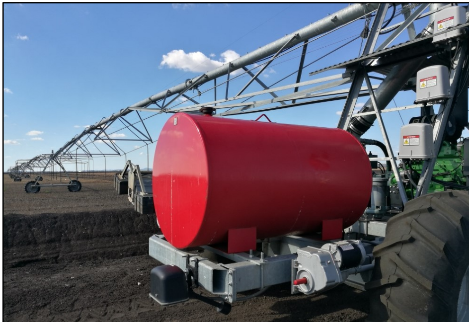
Figure 1-1: A diesel Gen-set LM irrigating a cotton field at Condamine Plains in southern Queensland, Australia
