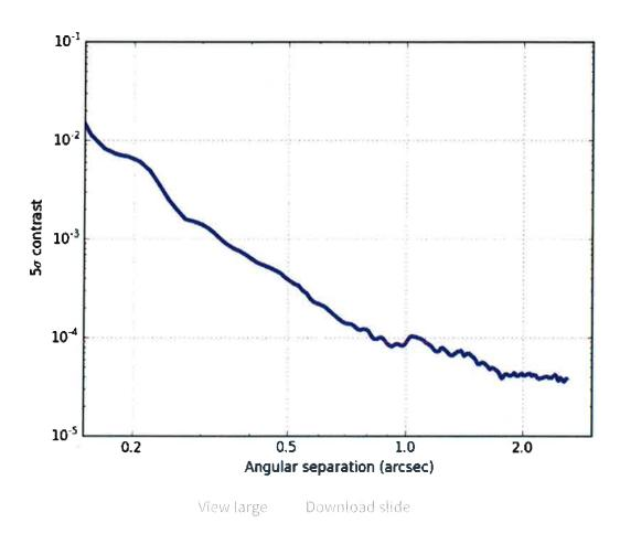
5σ detection limit as a function of angular separation derived from the NAOS-CONICA AO image around KELT-10. [A colour version of this figure is available in the online journal.]
